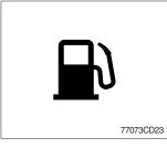
① This warning lamp lights ON when the fuel level is low. Refuel the machine as soon as possible.
