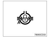
① This lamp lights ON when the differential lock function is operating.
